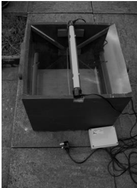
A "Skinner" type trap With 15w Actinic tube
